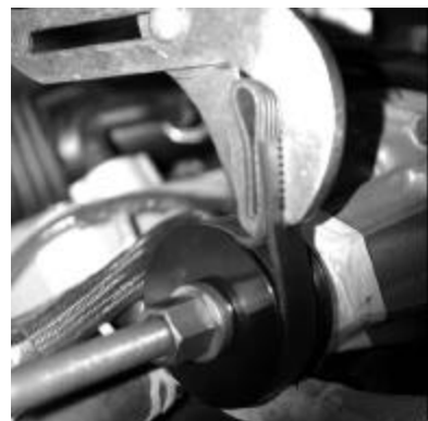
Using a section of old belt for a strap wrench to tighten or loosen the threaded rod.
