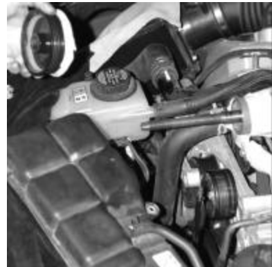
Leave the threaded rod attached to the supercharger.
